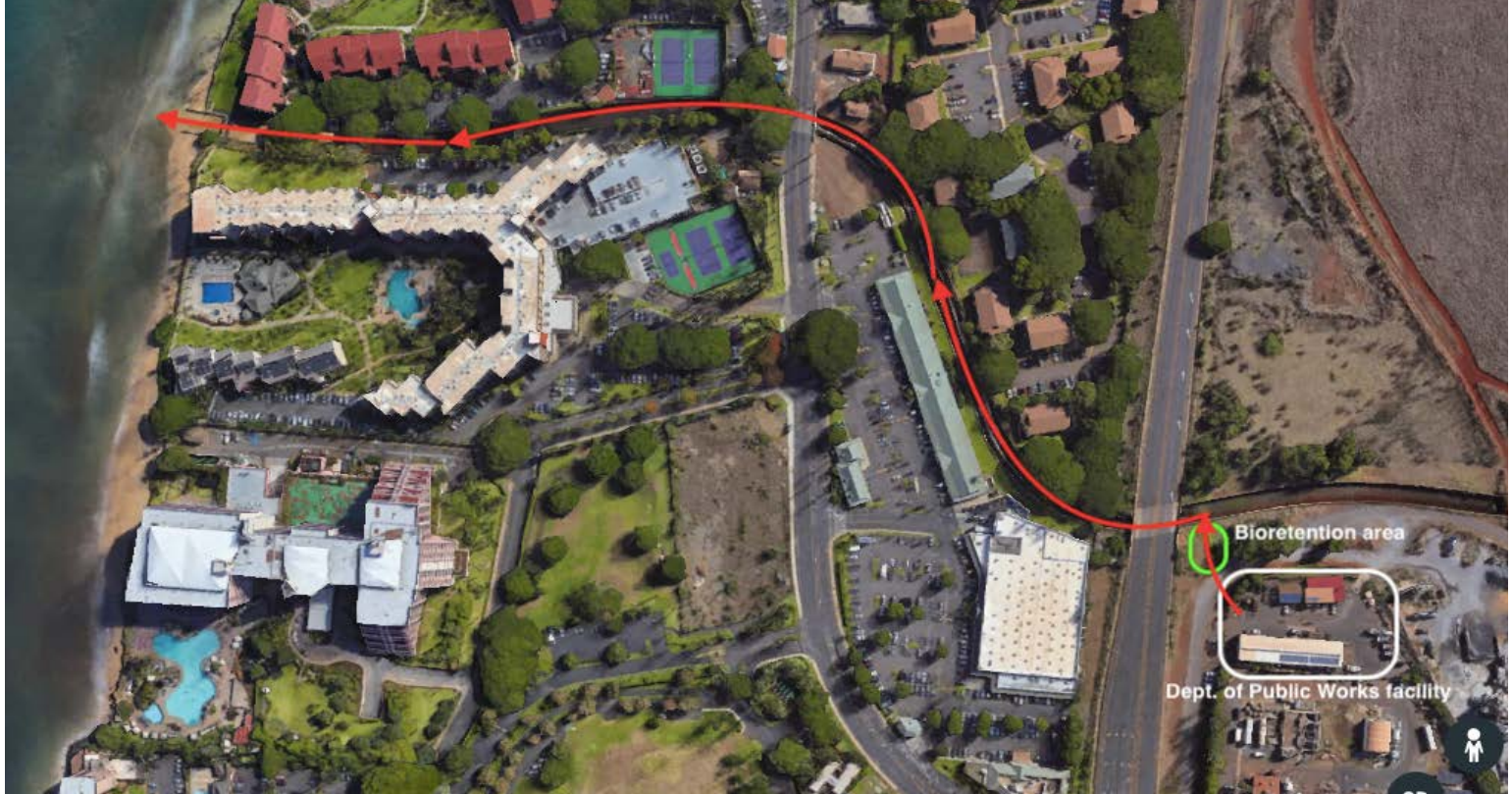
Path of runoff flow from the DPW Lāhaina baseyard facility, through the Honokōwai Gulch and into the ocean.
